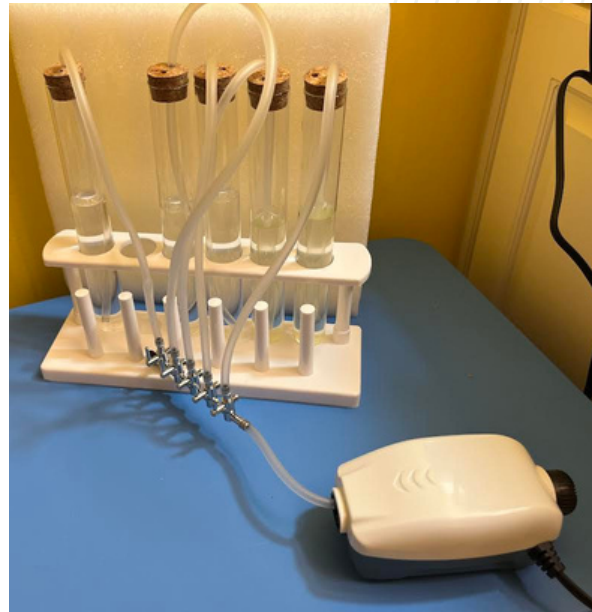
Figure B4. Pump to bioreactor connection
