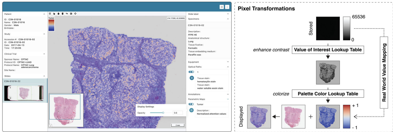
Fig. 8 | Display of saliency, class activation, or attention maps. Screenshot of the Slim user interface displaying an attention map image overlaid on the source slide microscopy images from Clinical Proteomic Tumor Analysis Consortium (CPTAC) project (upper left). The attention map was derived from the slide microscopy
